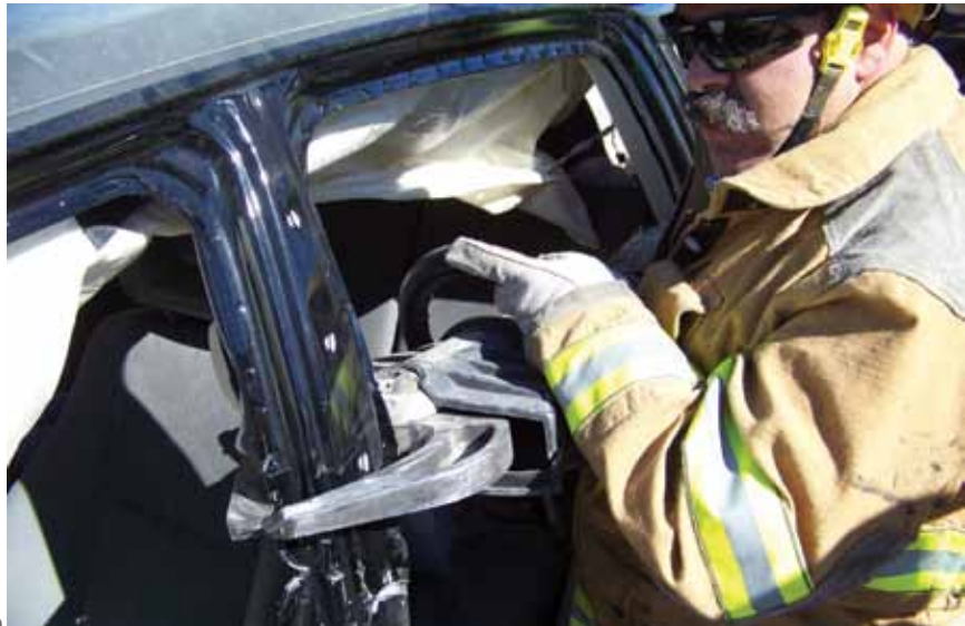
The most successful tool position for cutting through a Boron B-pillar was this "parallel" position. The blades were able to close more before cutting into the metal, letting them generate a greater force than if they were loaded while fully opened.
